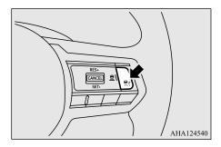
The display on the information screen of the instrument cluster will switch to show information on the ACC.
