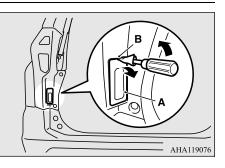
3. Pull out the service lid (A) in the direction of the arrow and remove the insertion part (C).
