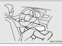
Deployment of front airbags and driver's knee airbag\*
