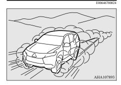
Check the sandy road condition and set the drive mode-selector to "4HLc" or "4LLc". Gradually depress the accelerator pedal to start the vehicle and drive at a possible constant low speed. Either set the Off Road mode-selector (if so equipped) to "SAND", or set the rear differential lock (if so equipped) to ON if the vehicle is likely to get stuck. This may help you drive smoothly.
