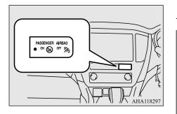
The indicator normally comes on when the operation mode is put in ON, and goes off a few seconds later.
