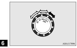
→: Turn the drive mode-selector while holding it down
