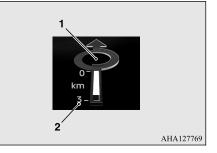
1- Guidance display Display the direction of vehicle travel and the guidance location.
