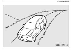
Set the drive mode-selector to "4HLc" or "4LLc" position, use the engine brake (down-shifting) and descend slowly.
