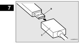
3. Connect the USB connector cable to the USB input terminal.
