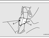
2. After the seat belt is retracted completely, insert the small latch plate (A) into holder (F), and then insert the latch plate (B) into the holder (F).
