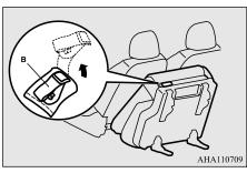
7. Securely retain the second seat by hooking the retaining bands onto the head restraint of the front seat and adjusting the length of the retaining band.
