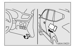
3. Open the fuel tank filler tube by slowly turning the fuel cap anticlockwise.
