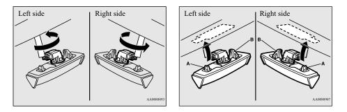
3. Remove the bulb by pulling out.
