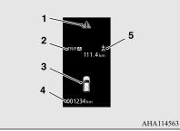
1- A mark display  $\rightarrow$  P.5-6 2-Information screen  $\rightarrow$  P.5-4 Interrupt display screen  $\rightarrow$  P.5-5 3-Door ajar warning display  $\rightarrow$  P.5-6 4-Odometer  $\rightarrow$  P.5-8
