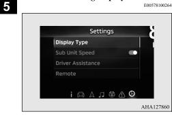
"Display type", "Sub unit speedometer", "Driver assistance", "Pop-up notification", "Rest reminder", "Turn-signal sound", "Operation sound", "Language", "Unit", "Factory reset", etc. can be changed to the setting of your choice.
