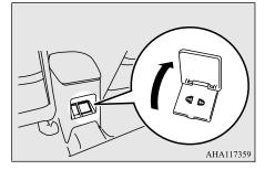
Insert the plug in the power outlet firmly. Make sure the plug is connected correctly.
