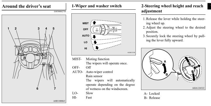
The washer fluid will be sprayed onto the windscreen by pulling the lever towards you.
