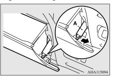
3. While pressing the side of the glove box, unhook the left and right hooks (B) and lower the glove box.
