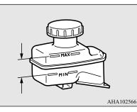
The brake fluid level must be between the "MAX" and "MIN" marks on the reservoir. The brake fluid level is monitored by a float. When the brake fluid level falls below the "MIN" mark, the brake fluid warning lamp lights up.
