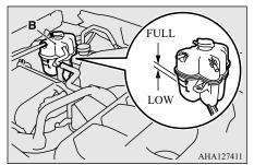
5. Add coolant to the radiator and/or reserve tank if necessary (refer to the "Maintenance" section).
