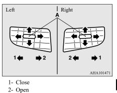
Adjusting the air flow direction
