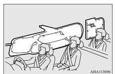
Deployment of side airbags and curtain airbags
