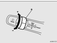
"+"- Higher sensitivity to rain "-"- Lower sensitivity to rain
