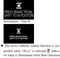
tor lamp is illuminated while these functions are suspended. It does not indicate a problem. When "2H" or "4H" or "4HLc" is selected, this lamp goes out and function again. Refer to "ASTC indicator lamp or ASTC OFF indicator lamp" on page 6-72.
