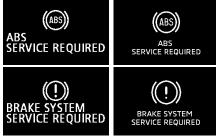
The ABS and brake force distribution function may not work, so hard braking could make the vehicle unstable.
