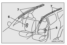
6- Side airbag modules\*7- Curtain airbag modules\*
