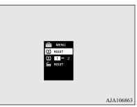
4. The warning lamp start flashing slowly.5. Drive for a while. The reset is completed if the warning lamp goes out.
