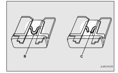
B- Fuse is OK C- Blown fuse
