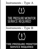
Each tyre should be checked monthly when cold and inflated to the inflation pressure recommended by the vehicle manufacturer on the tyre inflation pressure label. (If your vehicle has tyres of a different size than the size indicated on the tyre inflation pressure label, you should determine the proper tyre inflation pressure for those tyres.)
