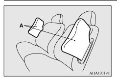
The label shown here is attached to the seatbacks with a side airbag.
