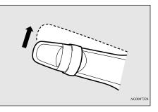
The wipers will operate once if the lever is moved to the "AUTO" position and the knob (C) is turned in the "+" direction when the operation mode is in ON.
