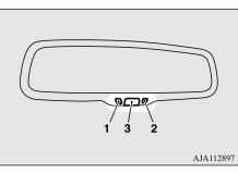
When the operation mode is put in ON, the green indicator (1) illuminates and the reflection factor of the mirror is automatically changed.
