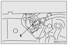
8. Insert the hexagon wrench into the hole where the plug was installed, and continue to turn it anticlockwise while pushing it in.
