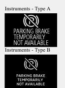
• If the parking brake indicator lamp blinks, the Electric parking brake cannot be applied. When this lamp continues blinking after waiting for a while, contact an authorised MITSUBISHI MOTORS dealer.
