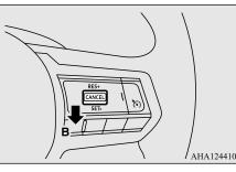
To slow down your speed in small amounts, push down the "SET -" switch (B) for less than approximately 1 second and release it. Each time you push down the "SET -" switch (B), your vehicle will slow down by approximately 1.6 km/h.
